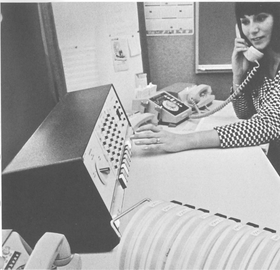
A variety of the most sophisticated communications equipment in existence is involved in POPS, HP's parts order processing system. Here Jennifer Bailes, central operator, works with a dataphone that links page-reading instruments at 23 company locations with Palo Alto's 360 computer, which prints out shipping instructions.
